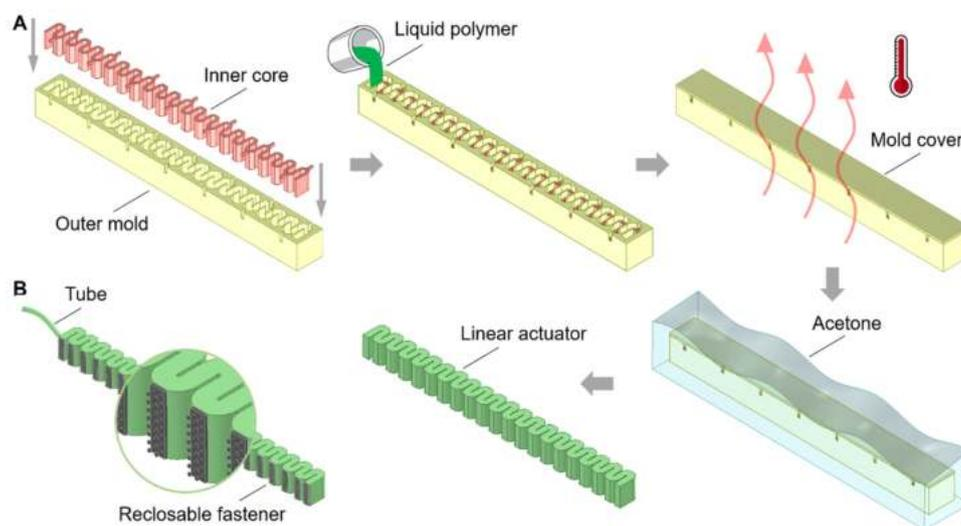
**Fig. 2.** Fabrication process of the DPSA. (A) Fabrication of the soft linear actuator. The outer mold and the inner core are assembled, the liquid polymer is poured, the liquid elastomer is thermally cured, and then the assembly is fully soaked in acetone to melt both the inner and outer molds thoroughly to obtain the soft linear actuator. (B) The RFs were bonded to each segment on one side of the linear actuator and a tube was attached to the actuator.
