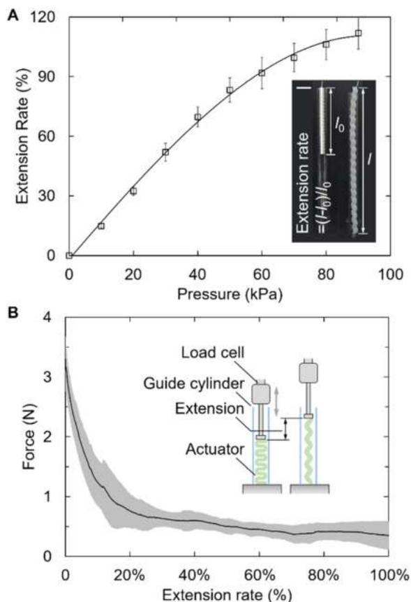
**Fig. 3.** Performance evaluations of the extending deformation. (A) The elongation of the DPSA (without substrate). The variable  $l_0$  is the length of the vertically hung actuator at 0 kPa, and  $l$  is the length of the extended actuator under pressurization. The inset shows the elongation of the DPSA at 90 kPa. (B) The linear blocking force of the DPSA (without substrate) at different extension rates. The inset shows the experimental setup. Scale bar: 30 mm.
